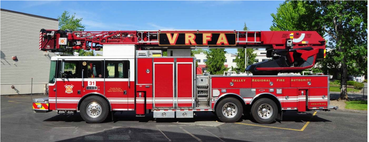
Valley RFA 2010 HME 1871 chassis by Rosenbauer, 102' Raptor Tower/Crane with body work by Metz 1500x300x20
