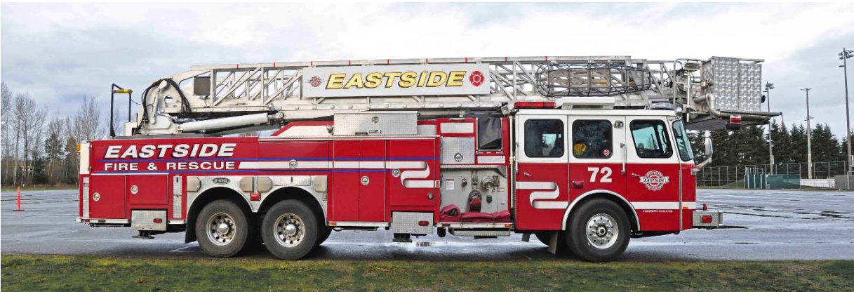
Eastside Fire & Rescue spare 2004 E-One spare platform with 2000 GPM pump
