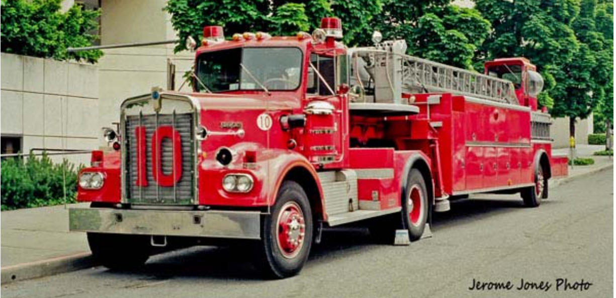
SFD Apparatus 315, a 1969 Maxim-Kenworth 100' aerial truck, with body work by Heiser. This workhorse was in service from July, 1969 until it was sold on April 8, 1994. Jerome Jones Photo
